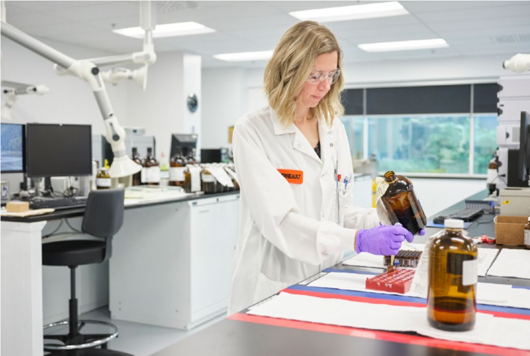
Joanie Perreault, Technician – Chemistry, Laboratory and Radiation Protection, is getting ready to analyse oil samples from a transmission substation.
