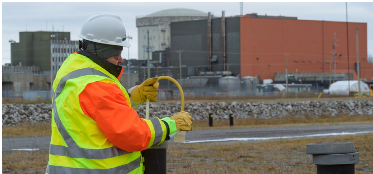
Photo taken as part of environmental monitoring at the Gentilly-2 facility. Here, a lab technician collects a groundwater sample from one of the many piezometers installed on site.
